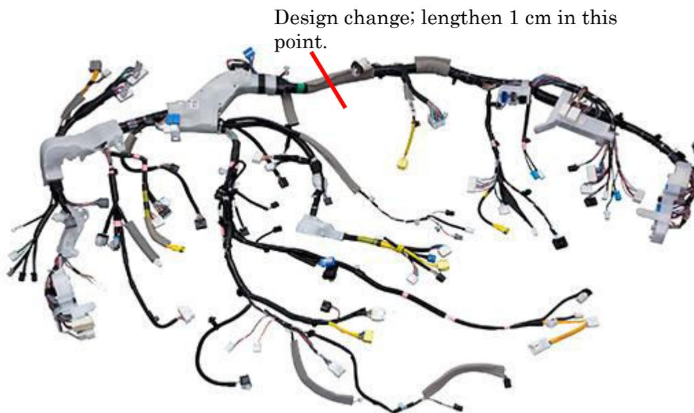
Design change which is related to the circuit length in the parts of trunk is worst case because all of the relevant circuits are required to change the length. As I wrote before all circuits are unique to just one part number or the car model. Of course this casual kaizen idea by the line worker relates to the cause of circuit obsolescence.
