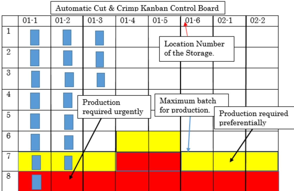
Above figure is the example of kanban control board for automatic cut & crimping machines. (And Hand crimping, Joint process were provided as well.)
