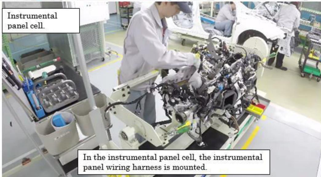
In the instrumental panel cell, the instrumental panel wiring harness is mounted.
