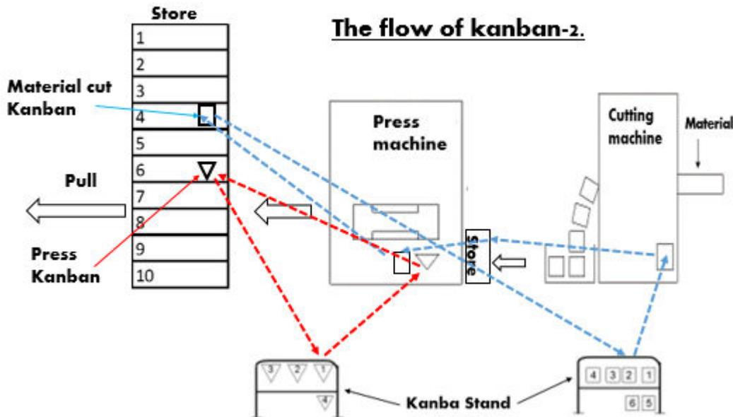
It is same production flow to “The flow of kanban-1”. But there is no [Store]. If the press machines and the cutting machine are very close, above kanban move is recommendable.
