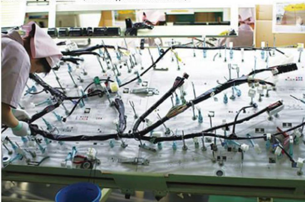
Wiring sub-assembly and circuits on the assembly board, Bundling with pvc tape, taping, putting protection parts (plastic protectors, corrugate tubes, pvc tubes---), putting clips and others exterior parts, visual inspection and electrical inspection. (And packaging.)
