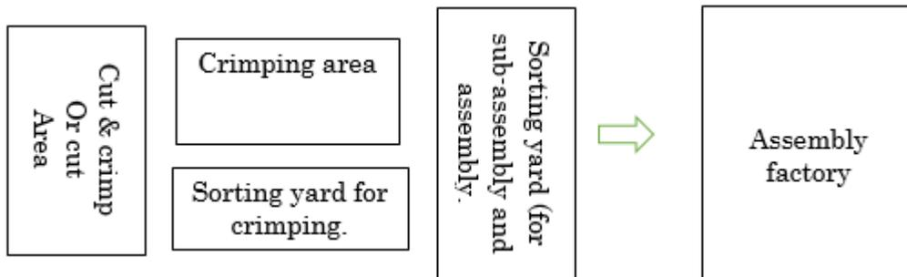
After cut & strip (insulation) & crimp if necessary to crimp in other end, the circuit is put in “sorting yard for crimp. And the circuits which finished the fabrication are put in the sorting yard (for sub-assembly and assembly).
