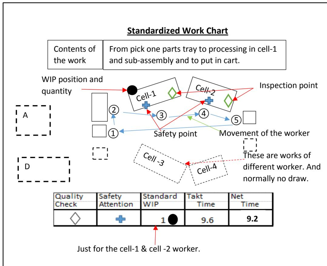
This is a very simple chart and standard. And any process in Toyota has this standard with working standard.
