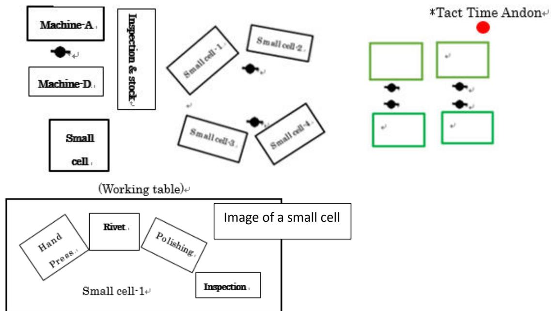
The process of the introduction of “Making stream of production” is next 5 activities. Seeking the Takt Time, Investigate the net-working time (Time study, Standardized Work Chart & Standardized Work Combination Table, Process Capability Table), Calculation of head account, calculation of necessary machine capacity (Process Capability Table, Standardized Work Combination Table), Move machines and Layout and Teaching & start.
