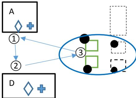
The supply carts have 10 trays each. Therefore for cell-1,2 there are 2 carts and 20 trays which means 20 sets of subassembly-1 (or subassembly-2) (as maximum stock). The requirement of the parts production is used the Double-Bin System which is one kind of primitive Kanban system. The rule is quite simple.
