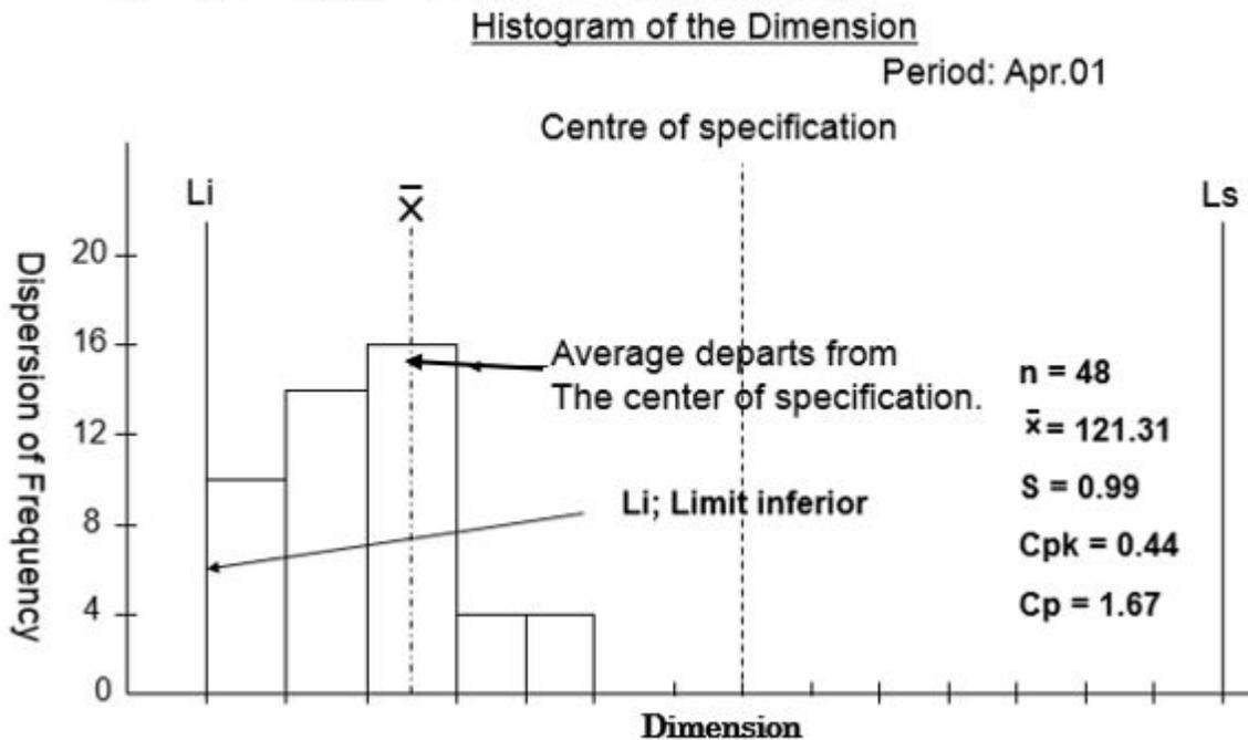
They made machine fine adjustment. However the defect trouble wasn't caused of the machine accuracy.
